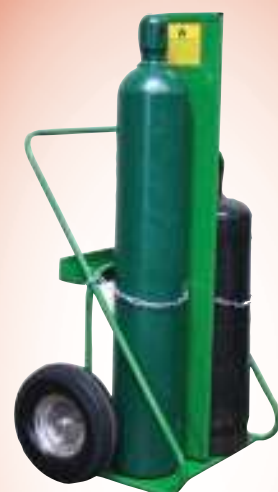
402-16FW Baseplate: 13" x 24" Height: 62" Width: 35" Weight: 118 lb. Wheels: SC-11B Cylinder capacity: 9.5" , 12.5"
